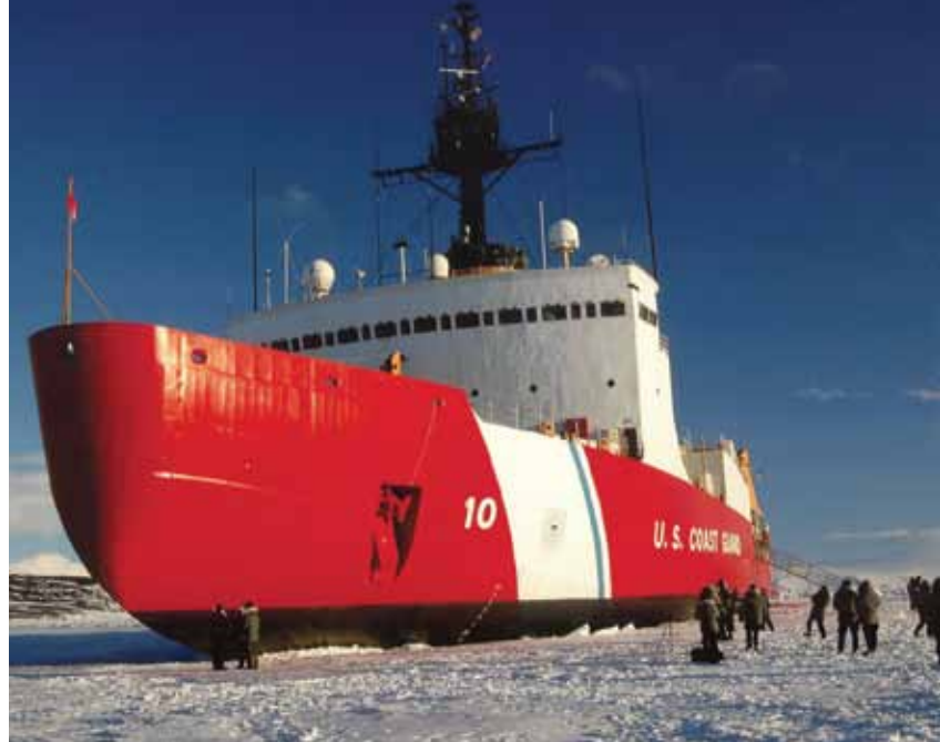
The upward angle of Polar Star's bow is designed so that the hull rides up onto the ice surface during icebreaking operations. (Photo from United States Coast Guard)
