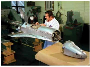
NASA model of space shuttle being prepared for testing in Langley's 16-foot Transonic Tunnel, May 3, 1978.
