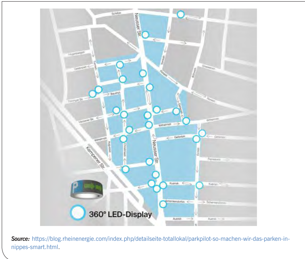
Figure 3: Locations of omnidirectional LED displays in the District of Nippes in Cologne
