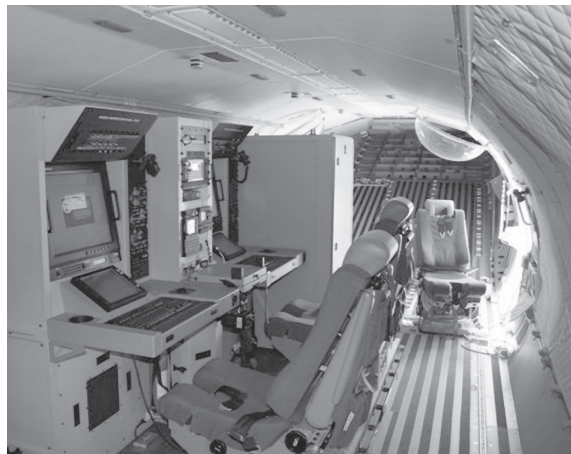
One of the features of the HC-144A aircraft is that its C4ISR components can be loaded and unloaded on transferable missionized pallets.
